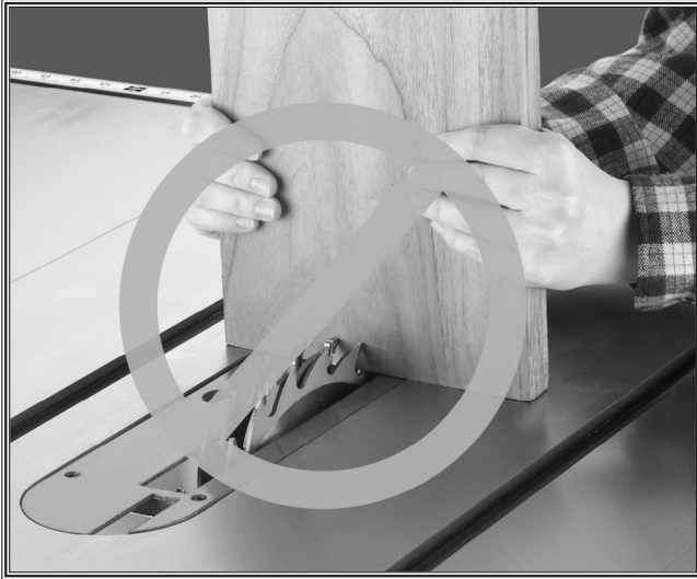
Figure 7. Do not make unstable cuts.
